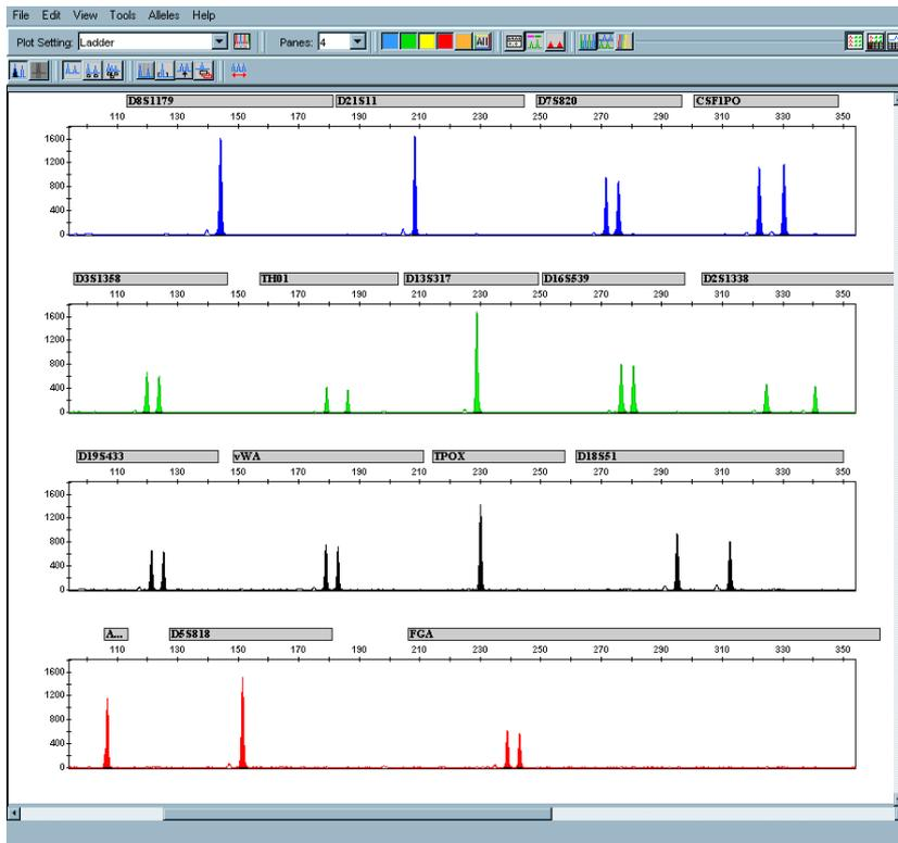
**Figure 1:** GeneScan® software electropherogram showing AmpFLSTR® Identifiler® PCR Amplification Kit results for 15 STR loci and the Amelogenin locus analyzed on the ABI PRISM® 310 Genetic Analyzer. DNA fragments are labeled in 6-FAM™ dye (blue), VIC™ dye (green), NED™ dye (yellow, depicted in black), and PET™ dye (red). The GeneScan™-500 size standard is labeled with LIZ™ dye (orange). Partial profiles are similar but missing information at some of these sites.
