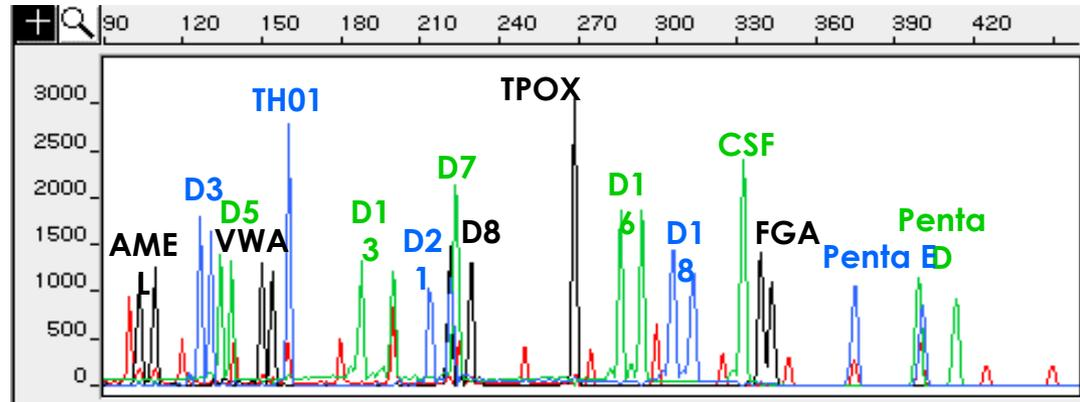
PCR Amplification with Fluorescent STR Kits and Separation with Capillary Electrophoresis
